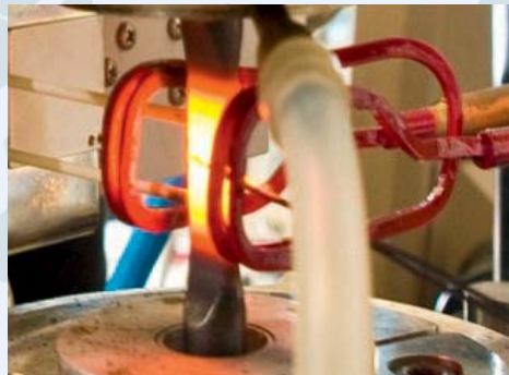
High-temperature fatigue testing of a Nickel-base superalloy
