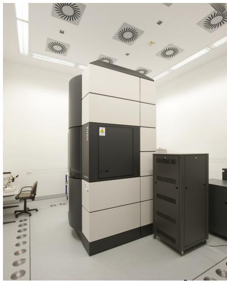
Fig. 1 The aberration-corrected Titan<sup>3</sup> 80-300 transmission electron microscope
